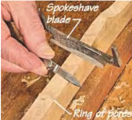
▲ Pic.5 The action of a wooden spokeshave is similar to a controlled knife blade
